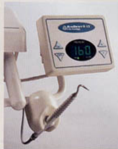
Figure 1 —The AirDent II CS control panel and handpiece installed next to the high-speed on the standard handpiece delivery system.
